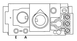
Figure 19. Pressure test points.
